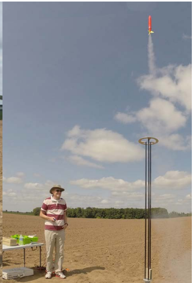
Taras Tataryn (foreground) and Saverio Prato preparing Taras' S2/P model for a pre-contest test flight. The egg "astronaut" is flown in the top payload section. The model is recovered by parachute. An onboard altimeter records flight data. / Pre-contest test launch of Peter Cook's S6A model.
