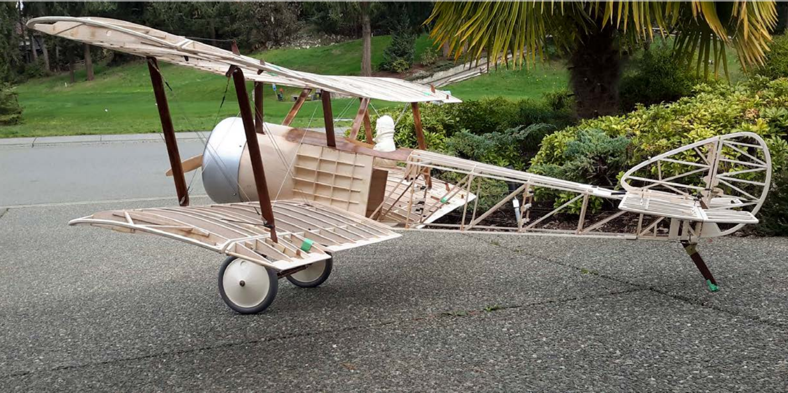
Brian Coolican's highly modified Balsa USA Sopwith Pup ready for covering. 108" wingspan, 32 lbs, Zenoah 80cc twin engine. Modifications include, steerable tail-skid, completely removable tail and custom wing tips. It will be covered with Koveral, two applications of Poly "C," then painted with latex paint. / Le Sopwith Pup (un kit très modifié de Balsa USA) de Brian Coolican est prêt pour l'entoilage. Spécifications : envergure de 108 pouces, moteur bicylindre Zenoah de 80 c.c. Les modifications comprennent un patin de queue dirigeable, un empennage amovible ainsi que des saumons d'ailes de construction artisanale.
