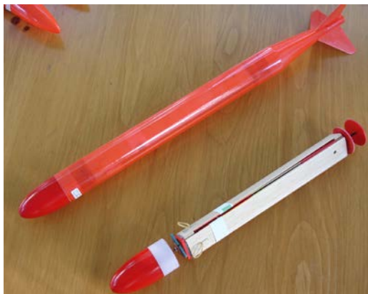
Peter Cook's S9A fiberglass carrier rocket (with gyrocopter loaded) and spare gyrocopter.
