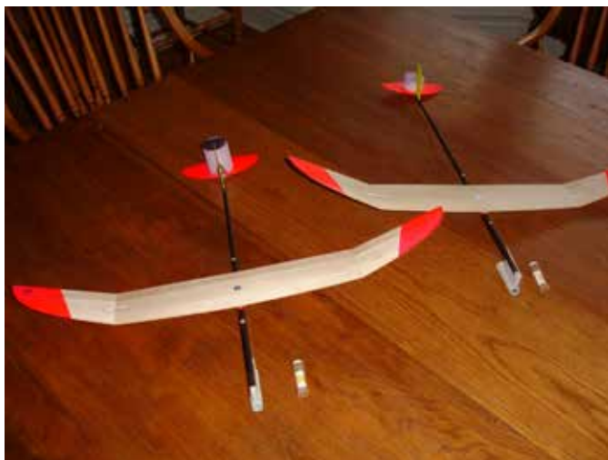
Close-up views of Peter Cook's S4A models. The wings fold and swing 90 degrees during engine boost. The 13 mm to 10 mm engine adapters used to mate the 10 mm diameter European engines into the 13 mm engine pod are also shown.
