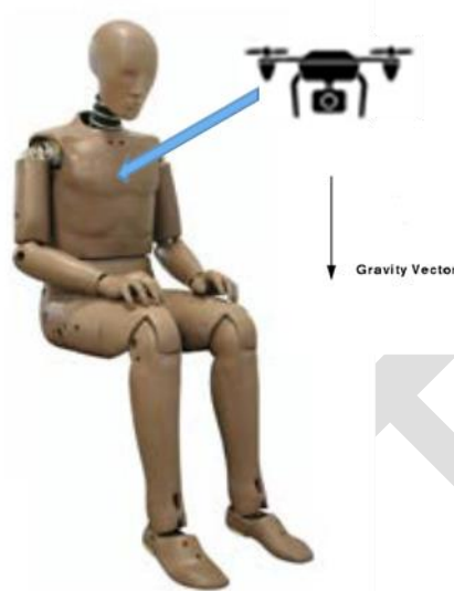
Figure C-5 – Chest Critical Impact Direction Test Configuration
